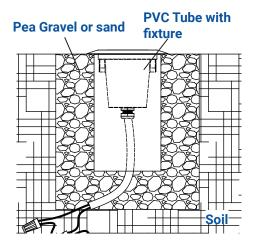
Install the PVC tube with the fixture in the hole and fill the hole with pea gravel or sand.
