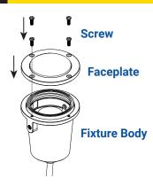
Place the lens and the faceplate back onto the fixture body and secure the removed screws in a star pattern using a screwdriver. Tighten until snug.
