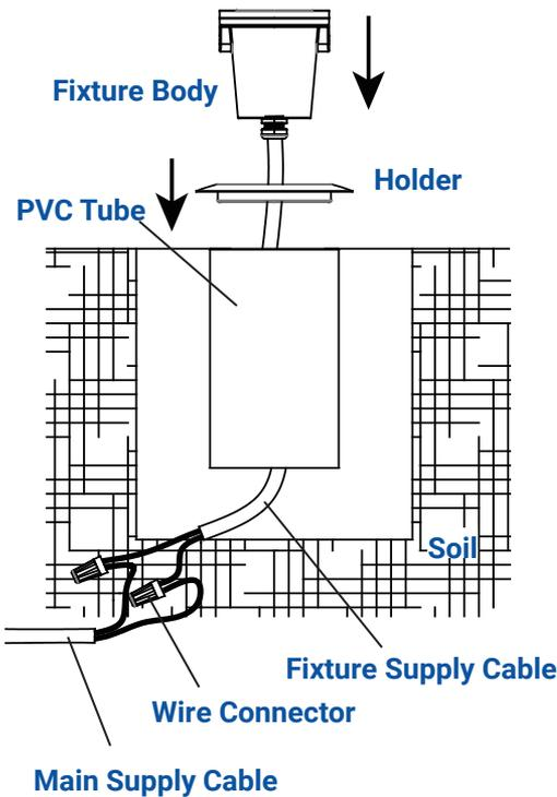
Pass the fixture supply cable through the holder and the PVC tube. Place the holder onto the PVC tube, then place the fixture body into the holder properly.
