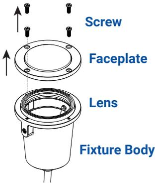
Use a screwdriver to loosen the screws on the faceplate and remove the lens from the fixture body.
