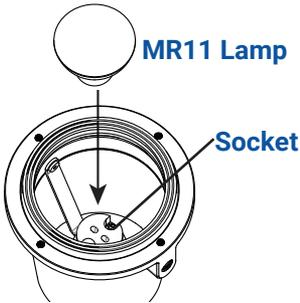
Insert the lamp with the correct wattage and type marked on the fixture label and push firmly into place.
