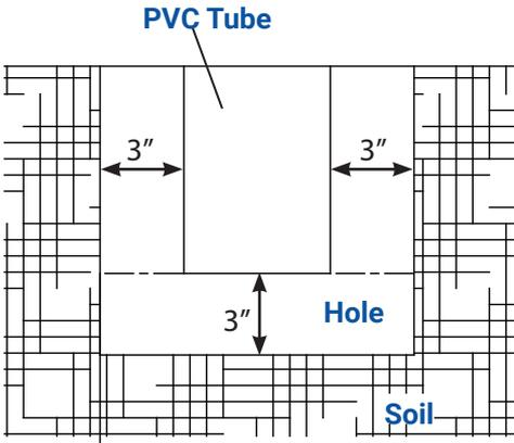
Prepare a hole in the ground. Make sure there are approximately 3" spaces surrounding the PVC tube for pea gravel or sand.
