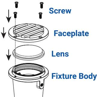
Place the lens and faceplate onto the fixture body and secure with previously removed screws in a star pattern. Hand tighten until snug with a screwdriver.
