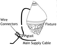
Strip both leads from luminaire pigtail. Using two wire connectors (sold separately), connect leads from luminaire to main supply cable leads.
