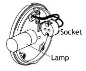
Insert lamp with the correct wattage and type marked on fixture label and push into place.
