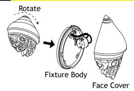
Rotate the face cover until it stops and then lift the cover straight off.
