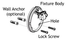
Attach the fixture body to your desired location and secure with lock screws.
